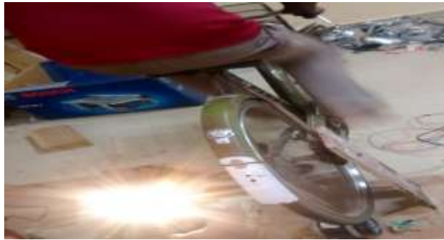
Fig.7 Lighting 45 watt DC bulb with pedal power
