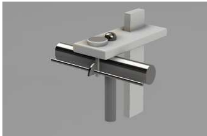
Fig.8 Schematic diagram of potentiometer set-up using CAD modeling
