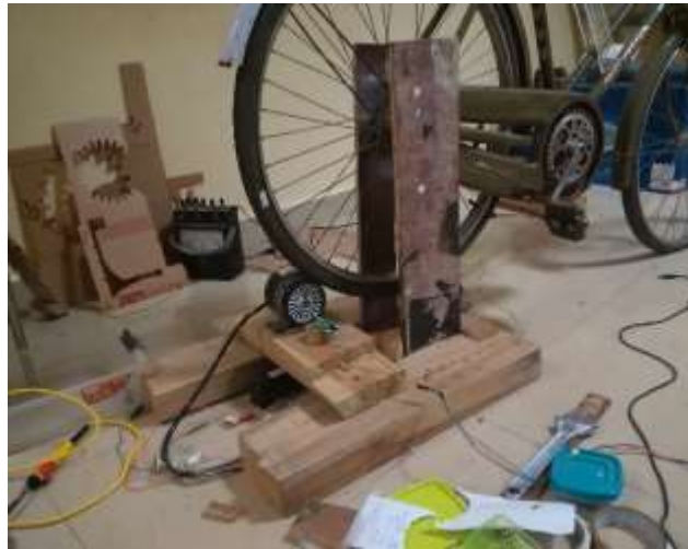
Fig. 3 Pedal power transmission mechanism
