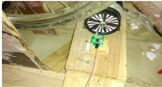
Fig. 10 IR sensor measuring acceleration and deceleration
